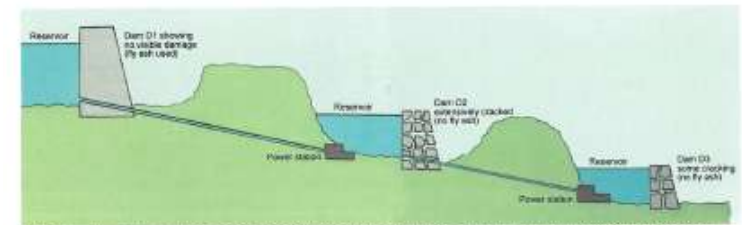
Fig 1: Schematic diagram showing the Cwm Rheidol Hydroelectric system, including the Nant-y-Moch Dam (D-1) and the Dinas Dam (D-2)
